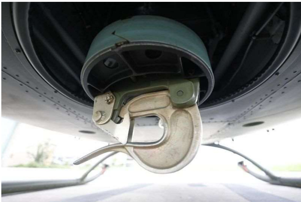
Figure 6.1: Factory Cargo Hook in “Hell Hole” viewed from below (UH-1H)
