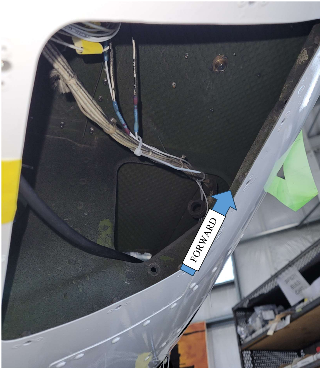
Figure 6.12: Cable to Side (on left side of rotorcraft belly)
