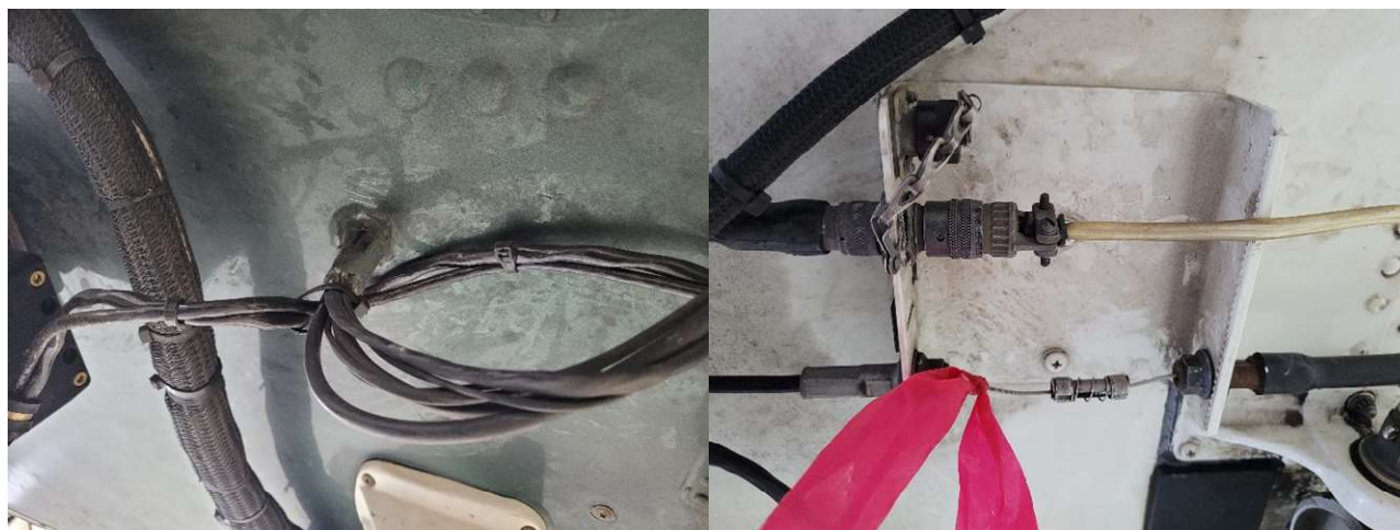
FIGURE 6.2: Right and Left pictures of Bell 407 Manual cable (206-072-902-005) and Electrical cable (Bell Ref. BHT-II-5, pg 10) shown as reference. Left image shows location of entry hole on 407 aircraft belly. FS and BL locations can be found BHT-II-5, pg. 7, figure 1-1, View E.
