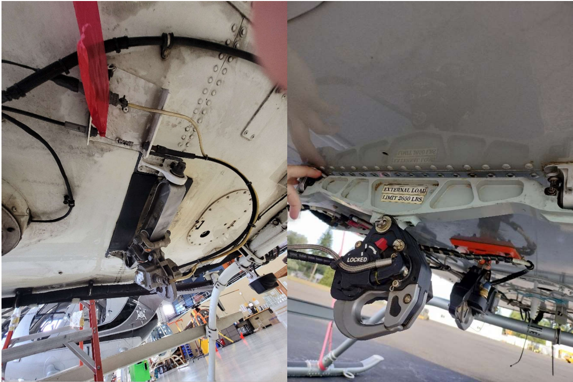
Figure 6.3: Examples of Bell 407 Cargo Hooks with Trolley (left) and Beam (right) Suspension Systems. NOTE: these are two examples of cargo hook kits available from Bell. For a complete list, see BHT-407-II-5 pg. i & ii.
